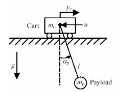
Fig. 3. Model of a gantry crane
