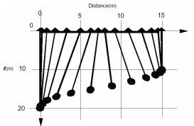
Fig. 6.Minimum time load transfer, smooth hoisting
