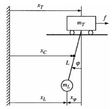
$m_{T,} m_{L}, L_{m}, x_{T}, x_{L,} \phi, f, g, x_{\phi} = x_{T} - x_{L} = L.sin\phi$  $x_{C} = (m_{T,} x_{T} + m_{L,} x_{L}) / (m_{L} + m_{T})$
