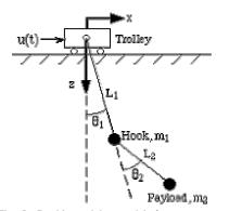
Fig. 5. Double pendulum model of a crane system
